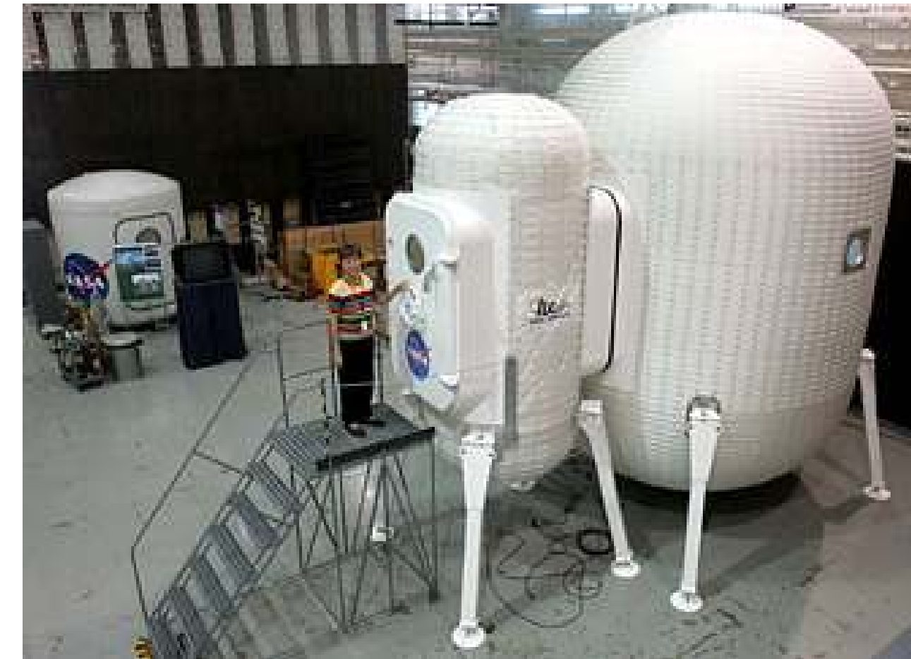
Model of an inflatable lunar habitat and airlock unit (sortie module) at one of the test and research centres
